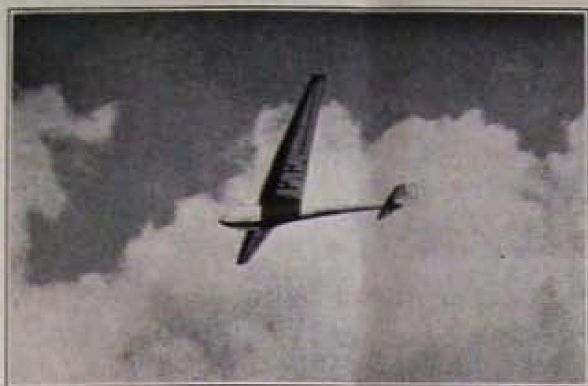
An "S-G 3" type sailplane flying in Poland. It is a full-cantilever cabin machine of 60 ft. span.
